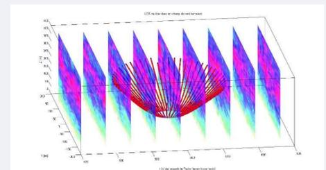
LOS for scanning lidar
