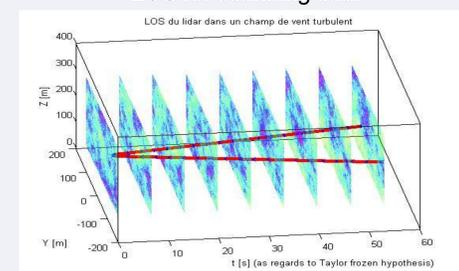
LOS for nacelle mounted Lidar
