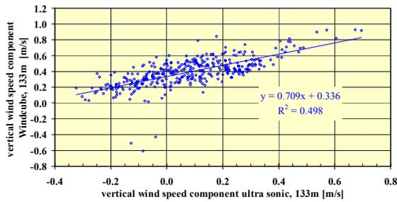
Figure 8: Comparison of vertical wind speed component measured at 133 m height above ground by Windcube and an ultra sonic anemometer (10-minute averages).
