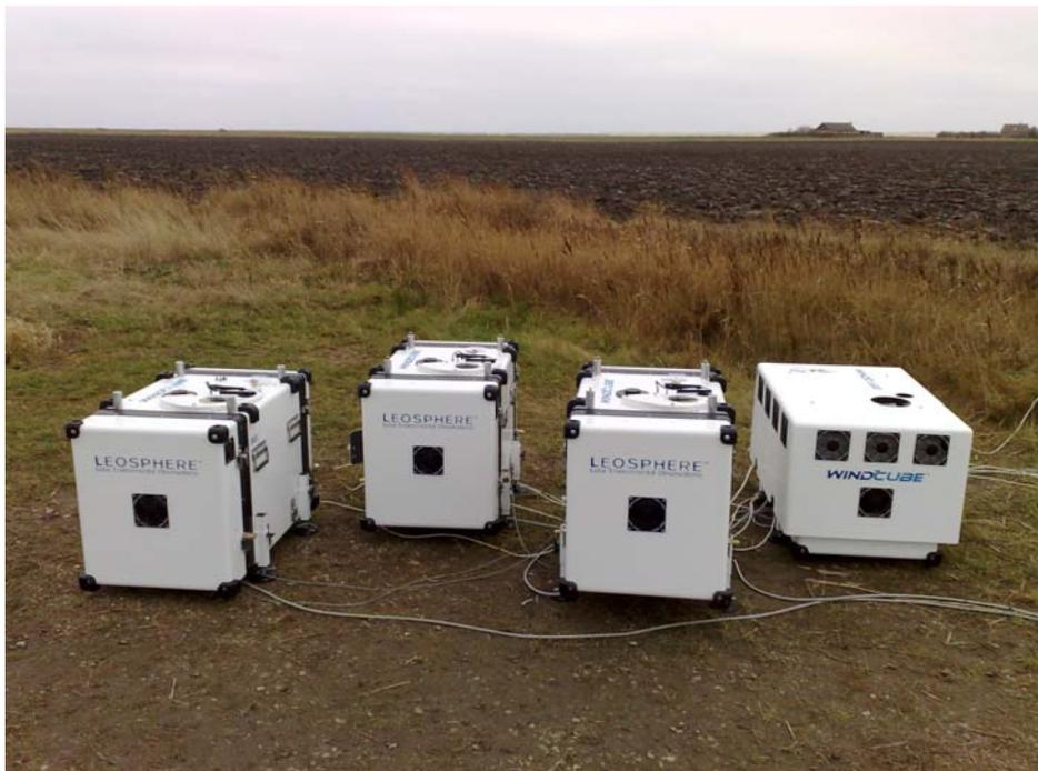
**Figure 2 Four Leosphere Windcubes on simultaneous test at the base of the meteorological mast at Høvsøre.**
